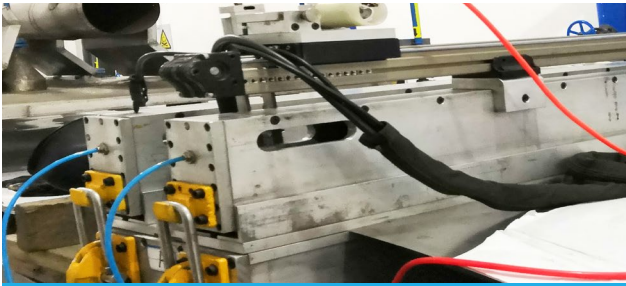
横向焊接 Cross welding
