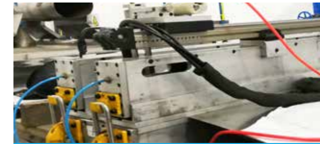
横向焊接 Cross welding
