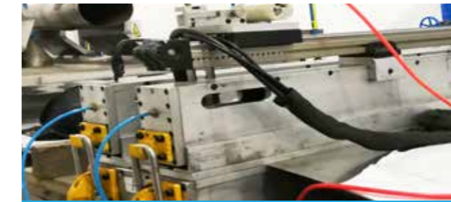
横向焊接 Cross welding
